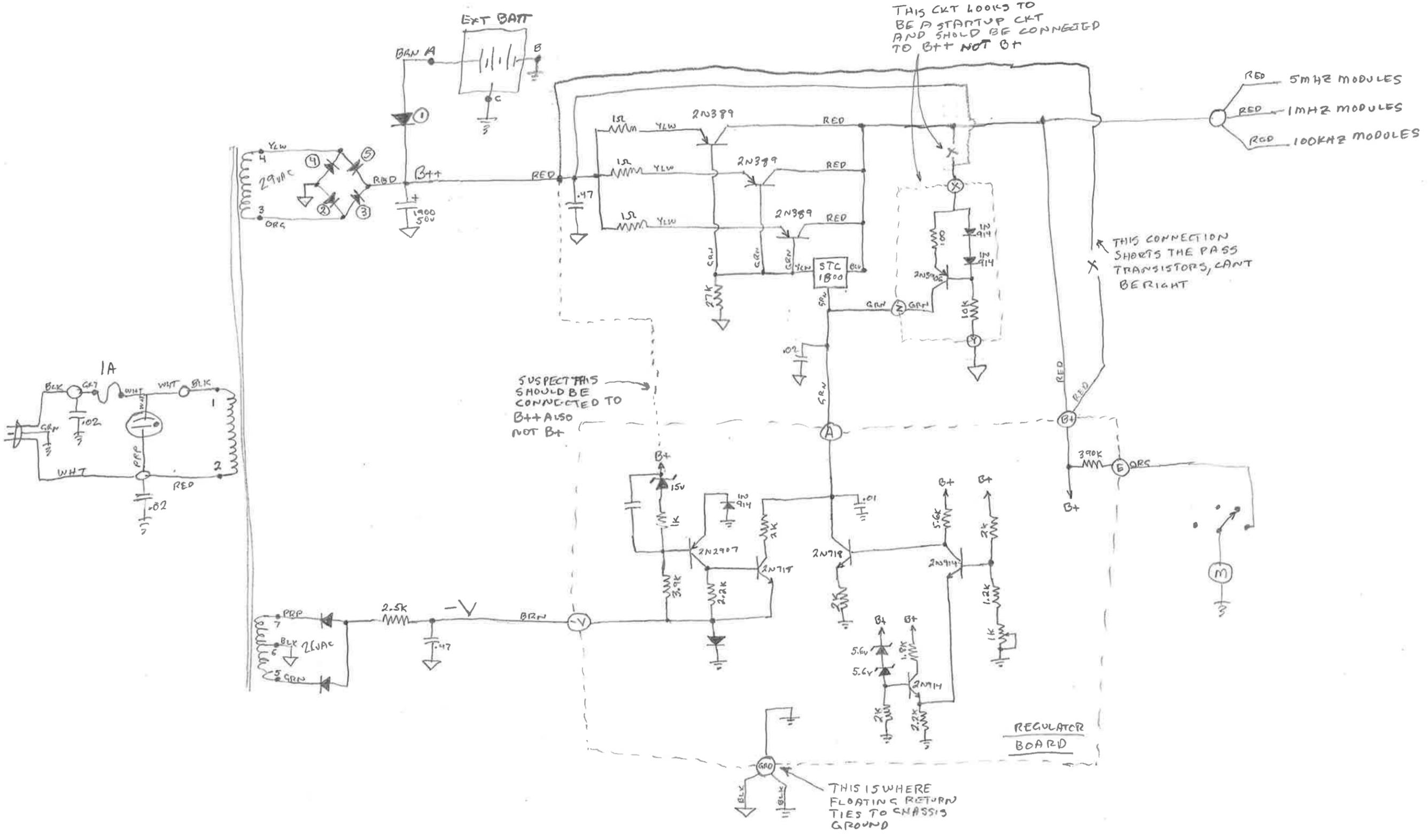
THIS CKT LOOKS TO BE A STARTUP CKT AND SHOULD BE CONNECTED TO B+ NOT B+
